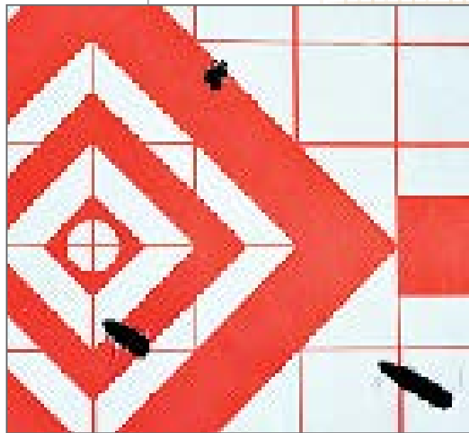
Example 24: Irregular hole in the lower right is a keyhole strike, which indicates a bullet stabilization problem.
